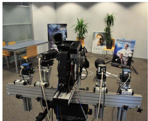
Figure 5. Camera rig for trifocal and structured light capture.
