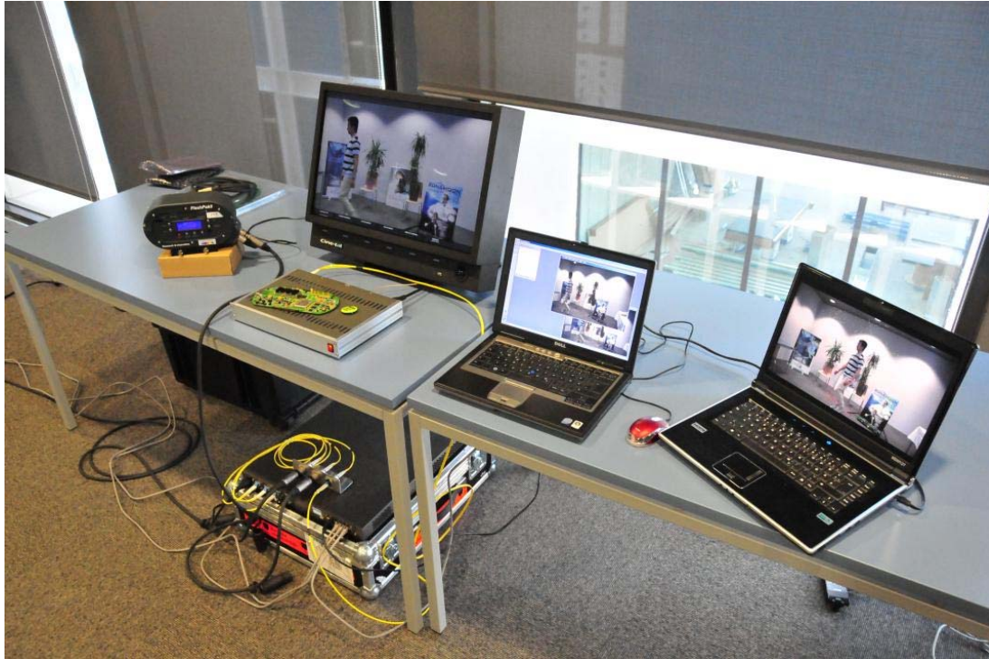
Figure 6. Capture infrastructure with FlashPakII recorder, preview monitor with 10G Ethernet converter box for the main camera, preview and control notebook for both two satellite cameras and notebook workstation for feature-point tracking (from left to write). The 10G Ethernet switch for stream routing is placed under the table.
